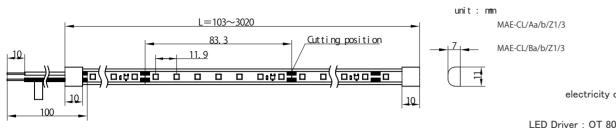
electricity consumption : 12W/m LED Driver : DC24V LED Driver : OT 80/220-240/24 DIM P The LED driver is sold separately.
